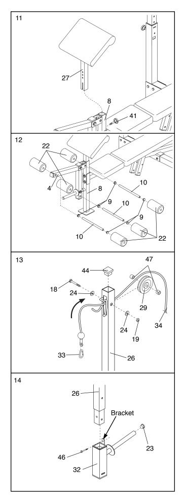
15. Secure the looped end of the Cable (34) to the M19 x 19mm Bolt (46) in the bracket on the Weight Carriage (32) with an M10 Nylon Locknut (19).
